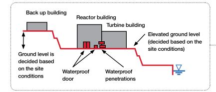
A number of countermeasures will be in place for the UK ABWR – these include a robust regulatory enforcement of site defences, to reduce the vulnerability to off-site impacts; revised consideration of site layout, such as positioning back-up buildings on higher ground; and increased safety-critical protection of emergency generation and back-up power systems, such as water-tight and impact-proof buildings.
