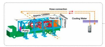
The UK ABWR will be equipped with increased on-site options to ensure cooling in an emergency, including on-site cooling vehicles, which can independently ensure the circulation of cooling water, and maintained cooling. These systems – which will be housed in protective buildings – can be attached to the station to ensure cooling is retained, even if primary cooling systems are lost and the site has no power.
